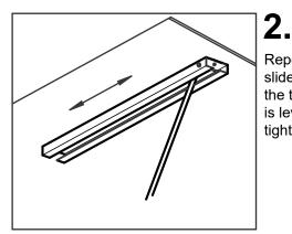
Reposition the slide bracket until the table top is level, then tighten screws.
