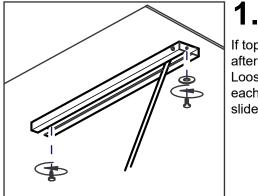
If top is not level after mounting -Loosen screws at each end of the slide bracket.
